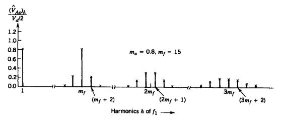
Fig. 4. Harmonic spectrum of Vo for sinusoidal PWM.
