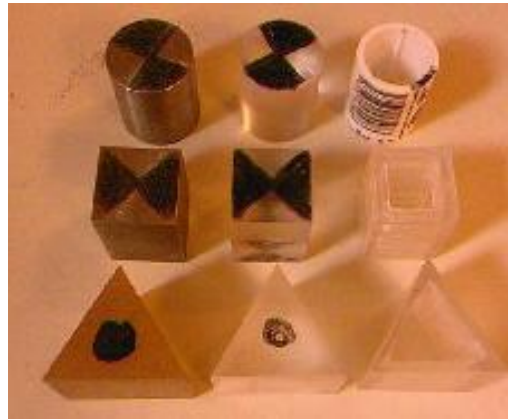
Figure 3.1: Free cells used in this study. From top to bottom: metal, PVC and hollow shapes
