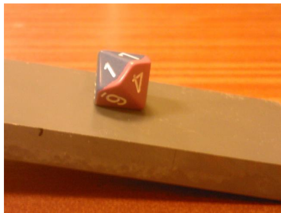
Figure 9.2: Measuring particle-wall static sliding friction of polyhedra.
