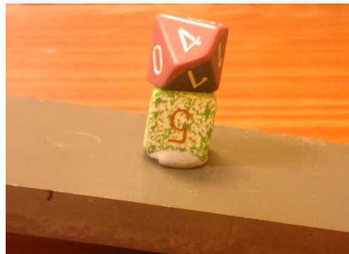
Figure 9.8: Measuring particle-particle static sliding friction of the polyhedra
