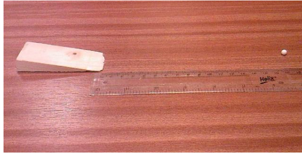
Figure 9.11: Measuring the particle-wall rolling friction
