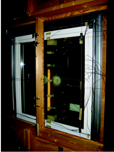
Figure 7 View of Frame A with glazing mounted in the hot box. The window is seen through an open door (which is closed during measurements) in the baffle panel on the cold (outdoor) side of the hot box. Thermocouples are used to monitor air and surface temperatures for the specimens.
