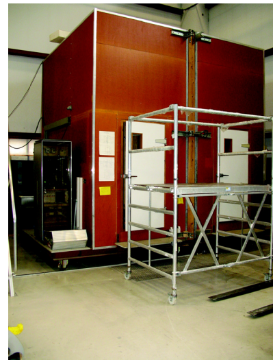
Figure 6 Hot box. The cold chamber is to the right and the warm chamber is to the left. The metering area of the hot box is 2.45 \times 2.45 m.
