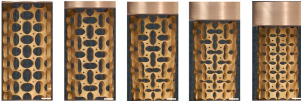
b) Brass specimen with PSF = 20\% under uniaxial compression
