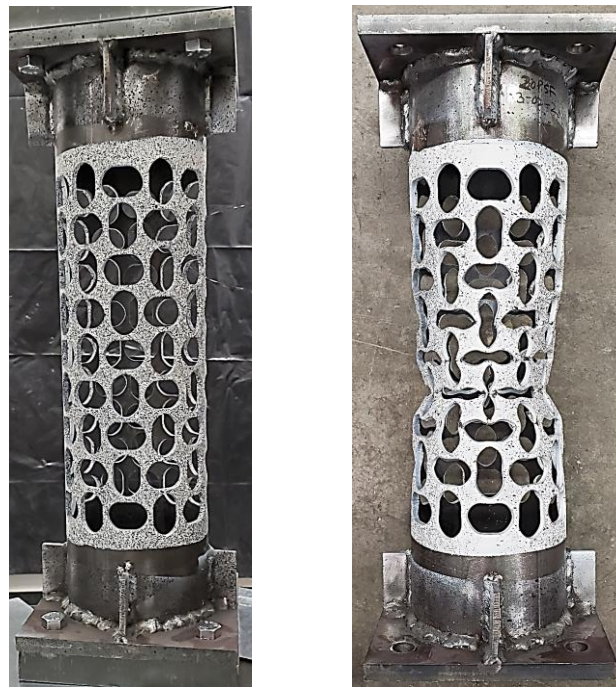
a) Prepared specimen b) Densification of tube
