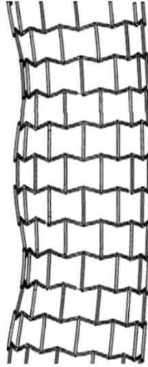
Figure 1.35: Rippled deformed shape for auxetic tubular structure under pure bending (Karnesis and Burriesci, 2013)
