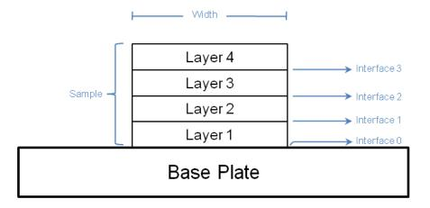
Figure 9. Sample welding interfaces
