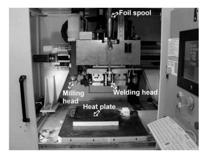
**Figure 2.** Solidica Formation<sup>™</sup> machine (as shown in [3])
