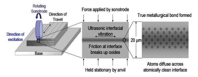
Figure 1. Schematic of the ultrasonic consolidation process
