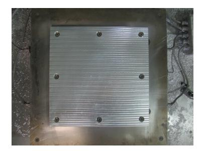
**Figure 4.** Geometry of the base plate used within the Solidica Formation<sup>™</sup> machine and bolt locations just before deposition
