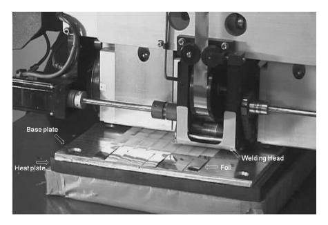
Figure 5. Base plate and part fixture in the Solidica Formation<sup>™</sup> machine
