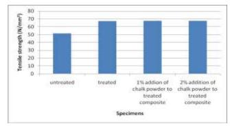
Fig.6. Tensile strength of specimens with addition of chalk powder
