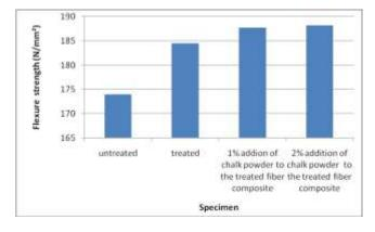
Fig.10. Flexural strength of specimens with addition of chalk powder.
