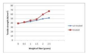
Fig.5. Tensile strength for varying fiber content
