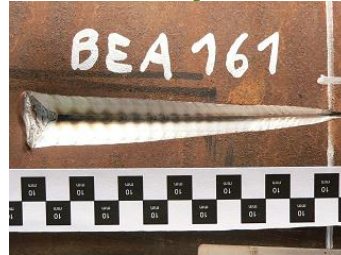
Dynamic, sharp tooth Deep gouge (single) Slower, worn tooth
