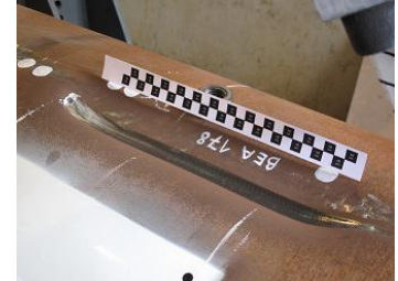
Dynamic, sharp tooth Deep gouge (single) Slower, worn tooth
