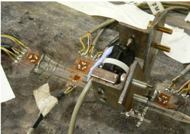
Defect 2.1.2 – Opening clip gauge
