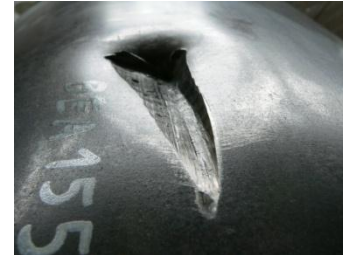
Dynamic, sharp tooth Deep gouge (single) Slower, worn tooth
