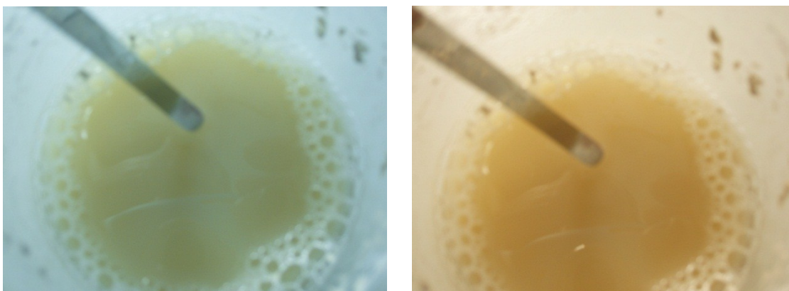
Figure 90: Photographs of 100 g calcium carbonate in a solution of 210 mg CTAB in 100 ml deionised water following full settling (top view)
