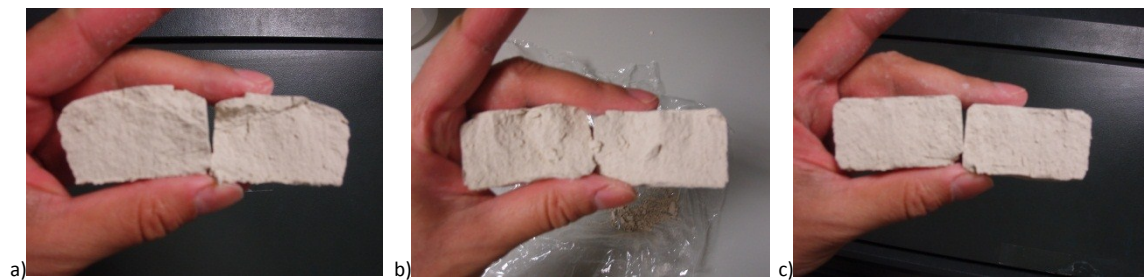
Figure 93: Photograph of filter cakes formed with Tween 80 surfactant a) 0.29 g/l; b) 5.12 g/l; c) 14.30 g/l
