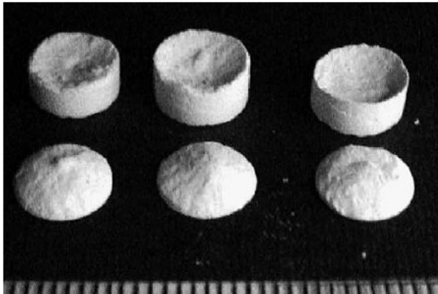
Figure 67: Photographs of broken tablets due to capping (Reference 190)
