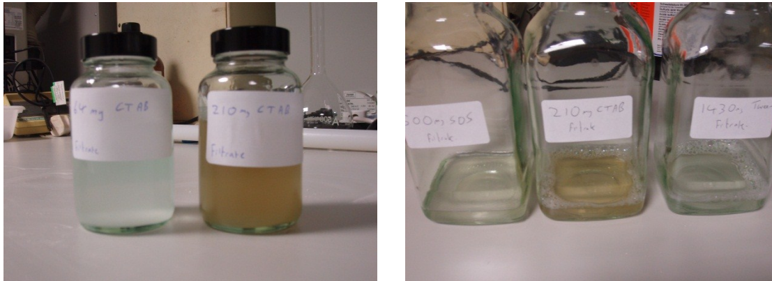
Figure 91: Photographs of a) 64 mg CTAB filtrate and 210 mg CTAB per 100 ml filtrate; b) SDS, CTAB and Tween 80 filtrate
