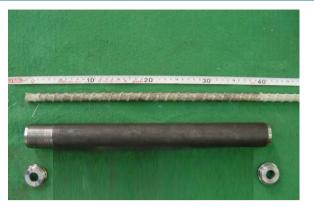
Figure 3. Steel adapter of FRP Hybrid Bars for tensile test.
