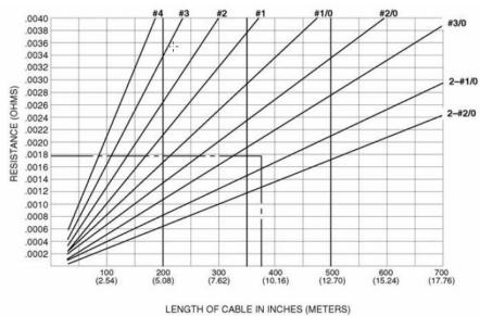
Resistance vs. length for various AWG cables sizes
