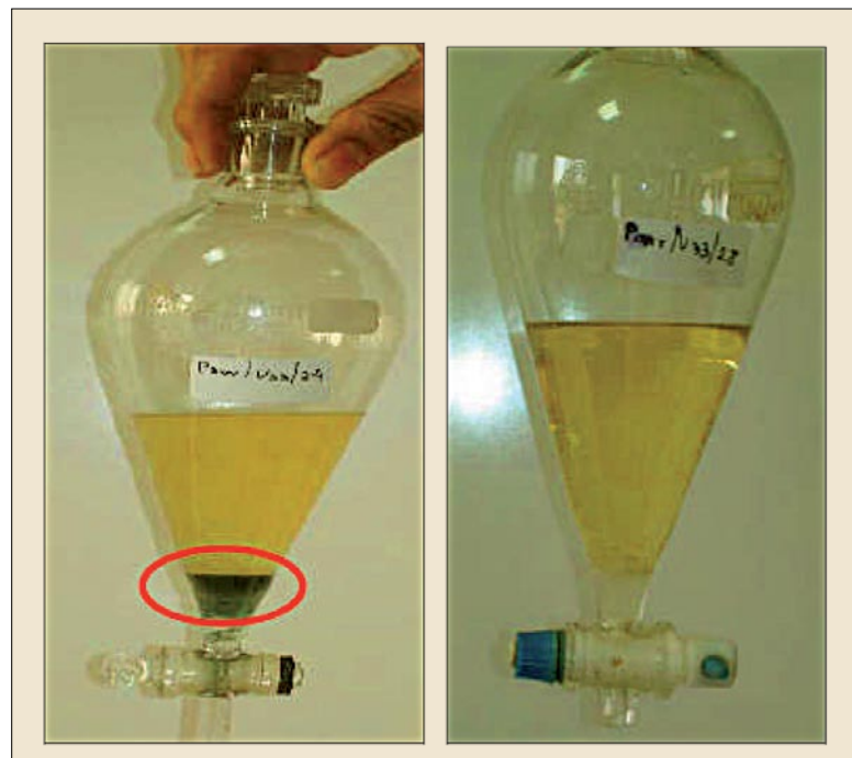
Figure 5 Black particles forming due to the presence of H_2S (left) and after treatment with Dorf Ketal additive (right)
