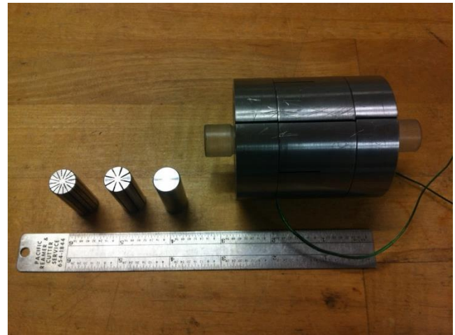
Fig. 5 Some of the machined armatures and coil sheath
