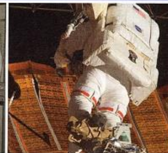
Dr. Parazynski, anchored to a foot restraint, prepares to work on a damaged solar array at the International Space Station.
