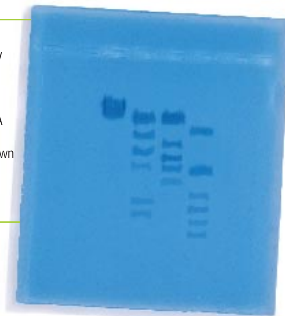
DNA samples electrophoresed in the Mini-Sub cell GT. Following a 30 minute run, 120 V, gels were stained with our unique Bio-Safe DNA staining solution. See the Electrophoresis Supplies Section for details on this new non-toxic DNA stain. Lane 1: uncut lambda ( \lambda ). Lane 2: Pst I \lambda digest. Lane 3: Eco R1 \lambda digest. Lane 4: DNA standard (Hind III \lambda digest).
