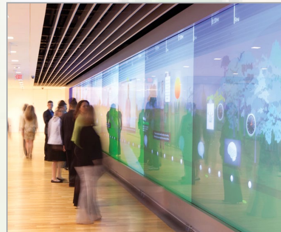
The Kaiser-Permanente 80'Wx10'H interactive videowall consists of eight rear-projection screens and eight projectors, which are programmed to allow the screens to act independently or as a single long mural.
