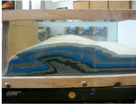
Above: Students crank the movable wall. After 20 turns of the crank they stop and observe the faults, measure the angles, and draw what they see. Then they crank another 20 turns. The photo on the right shows the results after about 60 turns, with a wedge with multiple faults. Six or seven reverse faults are clearly visible cutting across the colored layers. On the surface students can observe fault block mountains and uplift.
