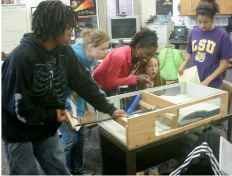
Above: Students crank the movable wall. After 20 turns of the crank they stop and observe the faults, measure the angles, and draw what they see. Then they crank another 20 turns. The photo on the right shows the results after about 60 turns, with a wedge with multiple faults. Six or seven reverse faults are clearly visible cutting across the colored layers. On the surface students can observe fault block mountains and uplift.
