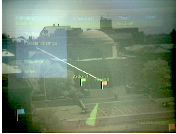
Fig. 6. An in-place menu realized with a screen stabilized menu and a leader line.
