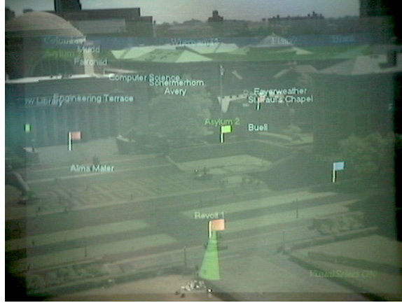
Fig. 1. A view through the mobile user's see-through head-worn display. (This and all other augmented reality images in this paper were captured by a video camera aimed through the see-through head-worn display.)
