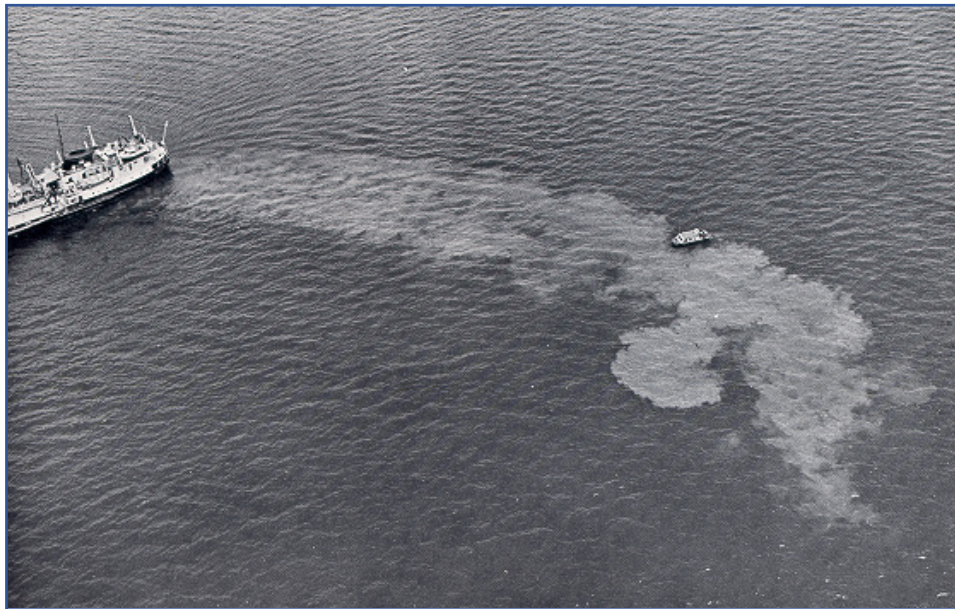
Figure 1. A hopper dredge discharging its load of sediment
