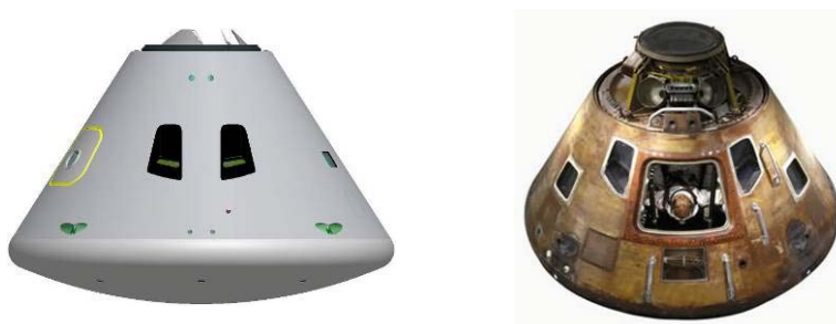
Figure 1: Shape comparison of a new crew module (left) and the previous Apollo capsule from the 1960's (right); not to scale.
