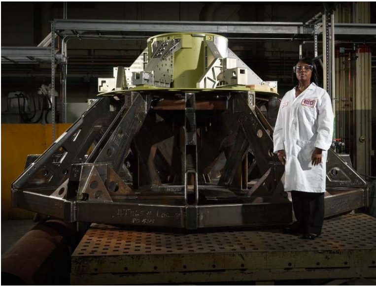
Figure 4: Parachute compartment atop the test vehicle structure
