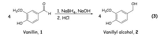
This preparation involves the reduction of the aldehyde group in vanillin (1, a flavoring compound found in vanilla) [See Note 1] to produce vanilly alcohol (2) using sodium
