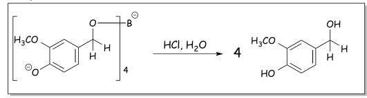
This addition of HCl (Step 7 in the Experimental Procedure) causes four reactions to occur:
