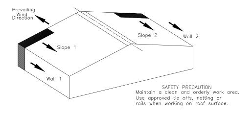
Install sidewall sheets first, beginning on the side away from the primary visual source, such as the rear wall of the building. This is will give you the best appearance. The roof sheets are installed last. Start the roof sheets so that the laps are away from the prevailing wind.
