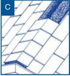
6.2.5 **Cobra® Exhaust Vent (hand nail version)** and **Cobra® Exhaust Vent (nail gun version)** have a ¾-inch or 5/8-inch nominal thickness, respectively, to facilitate ventilation. Care shall be taken not to crush or compact the product during installation. Figure D.
