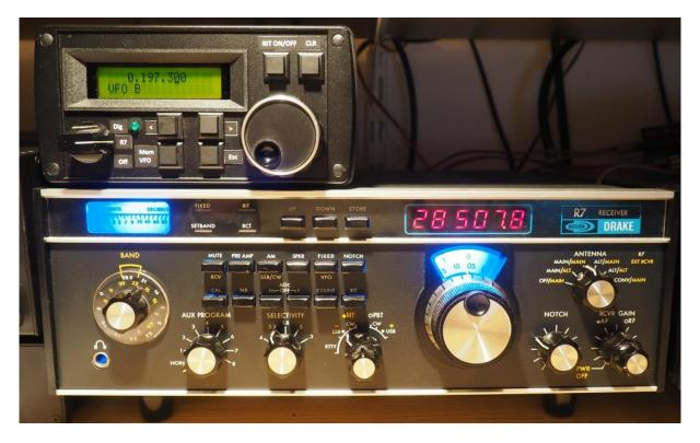
Picture 15: Dig. VFO B operates but doesn't control the R7
