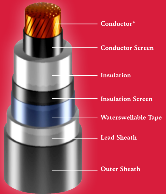
LEAD SHEATHED CABLE
