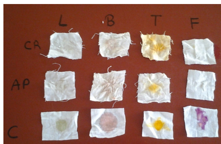
Fig 3.5: Stain removal with crude and partially purified protease
