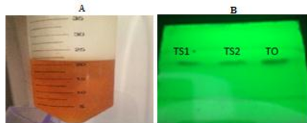
Fig. 2: (A): Thymus oil (B) TLC of Thymol at 252 nm (TS1) and (TS2) are standards (TO) Thymus oil
