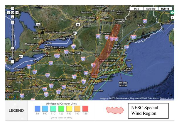
**Figure 1.** NESC Special wind region and coastal wind contours for New York and New England (map by TerraMetrics).
