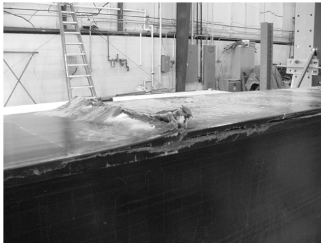
Figure 14: Typical compression flange failures for four-point bend testing of the 8" DWB (top photo) and the 36" DWB (bottom photo).
