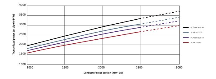
1) Assumed data: ambient temperature 15°C; burial depth 1.5 m; spacing between cables 20 m; soil thermal resistivity 0.8 m K /W
