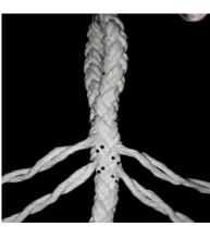
10) Note that all strand pairs have been tucked once now. The left-laid strands should all exit the rope on the same side. The right-laid strands should exit the rope 180° around the circumference from the left-laid strands as shown in picture on left.
