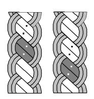
8) Tuck the marked leftlaid strand pair that is furthest from the eye first (shown on left in dark gray). Tuck under the right-laid strand pair on the standing part, so that it runs parallel to the marked, left-laid strand pair of the standing part (shown on right in dark gray).
