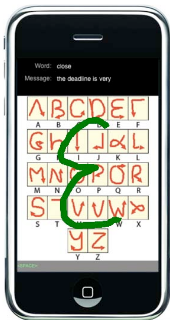
Figure 1. Text entry interface for eyes-free input. The stroke map is enhanced for clarity.
