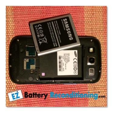
**Step 3:** Locate the polarity markings on your phone battery.
