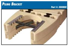
Allows lateral position adjustment to piles from 6'' (15cm) to 18" (46cm) in diameter. SS hardware.
