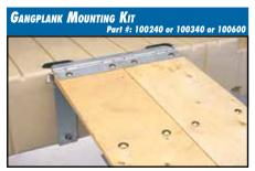
Galvanized steel hinge bracket and hardware, for wood walkways 24" (61cm), 34" (86cm), or 60" (1.5m) wide. Kits include hardware connectors with nuts, hinge-to-float bracket, hinge-to-plank bracket and 2 gangplank stiffeners with carriage bolts, nuts, and washers. Lumber not included.
