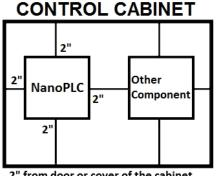
Provide the maximum possible <sup>2" from door or cover of the cabinet</sup> physical separation between solid state and electromechanical controls. If possible, the electromechanical controls (motors, starters, solenoids, etc.) should be housed separately or at the farthest point when enclosed within the cabinet. We recommend that the NanoPLC have a minimum clear space of 2" on all sides for adequate ventilation as shown in the image on the right.
