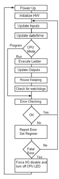
A good understanding of the NanoPLC's CPU operating sequence will help you achieve the proper control for your equipment or process. The flow chart on the left shows how the CPU controls all aspects of system operation.
