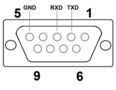
PGMCBL: NanoPLC Programming Cable Wiring
