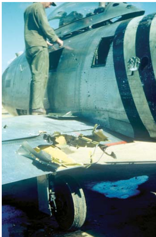
The MiG-15's 23mm and 37mm HE cannon shells could do substantial damage when they hit, but the F-86's robust construction could absorb a lot of punishment. Here, Maj Curtis L. Utterback's F-86A is shown after it was hit in the left flap. (Dean Juhlin via Warren Thompson)
