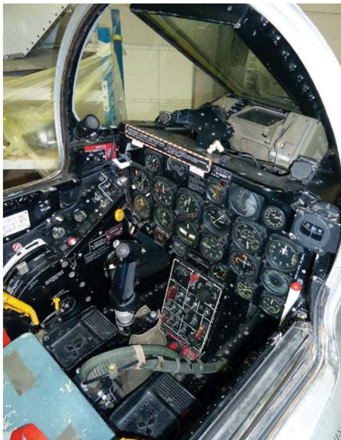
The Sabre "jock's" "front office" – the cockpit of an F-86A-5. The olive-colored apparatus mounted atop the glare shield is the A-1C(M) gunsight, projecting its reticule on the angled "combining glass" above it. (Duncan Curtis)
