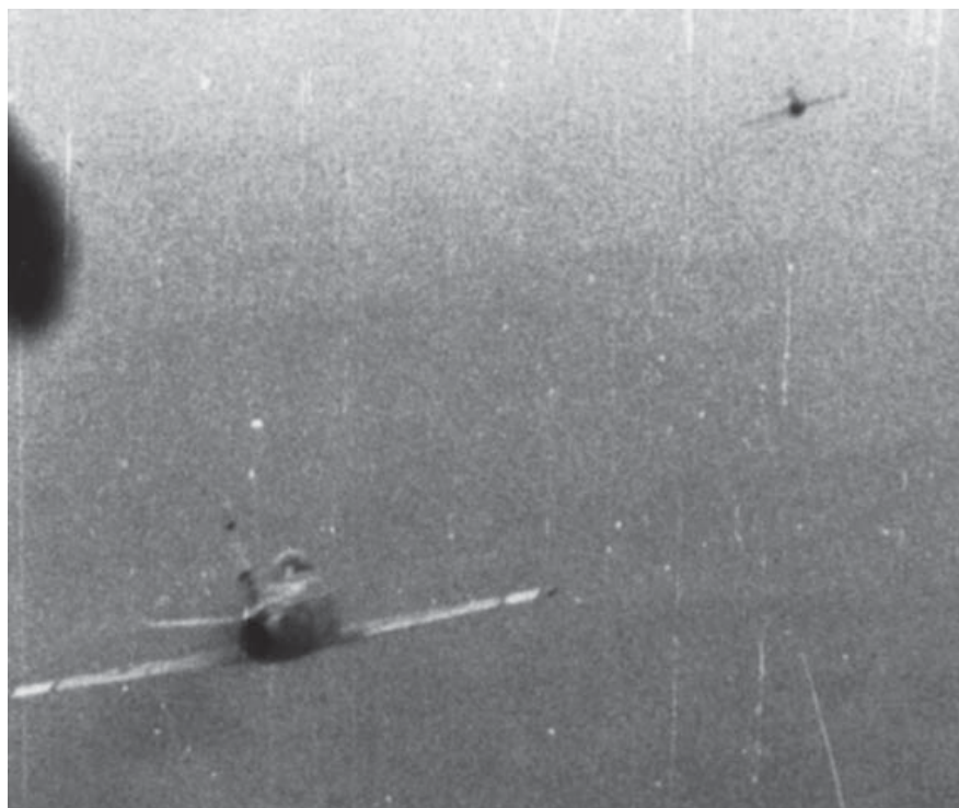
Lt Col Jones' wingman's view of the chase. Although not Pincoski's gun camera film, this frame illustrates the relationship of the two Sabres in "hot pursuit" of the MiG. When the trigger on the F-86's control stick grip was pressed to the first detent, the gun camera was turned on – pressing to the stop fired the guns. The wingman here is not shooting bullets past his leader to get the MiG, he's just filming it. [Larry Davis]
