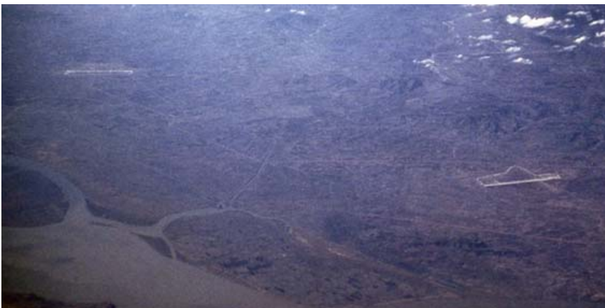
Just beyond the Yalu River, the Chinese rebuilt the former World War II Japanese Army Air Force airfield at Langtao (lower right), near Andong, with a jet-capable 6,000ft-long concrete runway and hard-surfaced taxiway in December 1950, and the brand new Dadonggou (upper left) airfield in May 1951. The Soviets based the 324th IAD at Langtao and the 303rd IAD at Dadonggou. (Dick Petercheff via Warren Thompson)
