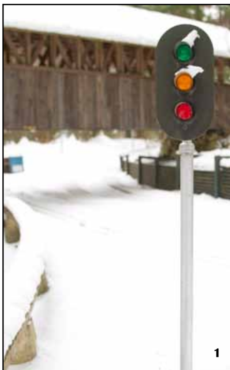
This Color Light signal is dark. A dark signal indicates STOP.
