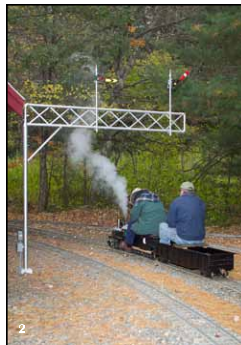
Signal indications on a Semaphore signal are read by the blade position by day and by colored light by night.
