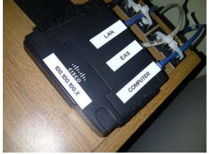
In addition, we put strain reliefs on the cables. We have found that many RJ 45s will release if too much force is applied to the cable. This will prove to be valuable in an environment where daily handling of the equipment is common.
