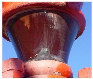
Arc tracks and cracks are visible on the surface of the insulator
