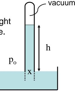
Since the density of mercury depends on the temperature, and the pressure reading depends on density, for accurate readings of atmospheric pressure this must be corrected for the local temperature.
