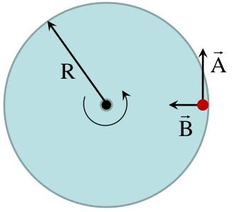
Since there is an angular acceleration  $\alpha$  the red spot has a linear acceleration tangential to the rim along  $\vec{A}$  that has magnitude,
