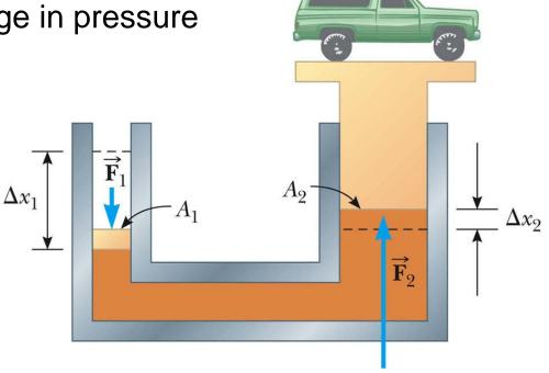
So the output force is the input force, times the ratio of the piston areas.
