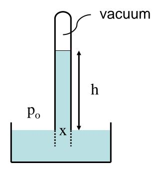
Taking h = 0 as zero pressure (absolute) the height of the fluid column is proportional to the pressure.
