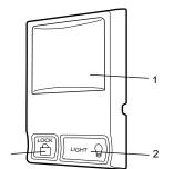
To turn off, press and hold the Lock button again for 2 seconds. The push bar light will stop flashing. The Lock feature will also turn off whenever the "LEARN" button on the opener panel is activated.
