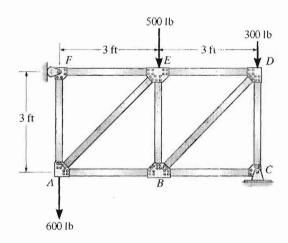
$$\Delta_{B_{v}} = \Sigma N \left(\frac{\partial N}{\partial P}\right) \frac{L}{AE} = \frac{1}{AE} \left[ (-600)(0)(3) + (848.5)(0)(4.243) + (-1100)(0)(3) + (1.414P + 1555.6)(1.414)(4.243) + (-(P + 1790))(-1)(3) + (-(P + 1400))(-1)(3) + (-(P + 1400))(-1)(3) + (-(P + 1700))(-1)(3) + (-(P + 1700))(-1)($$
