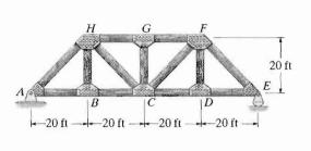
\*6-52. Draw the influence line for the torce in member HC, then determine the maximum live force (tension or compression) that can be developed in this member due to a uniform live load of 800 lb/ft that acts on the bridge deck along the bottom cord of the truss.
