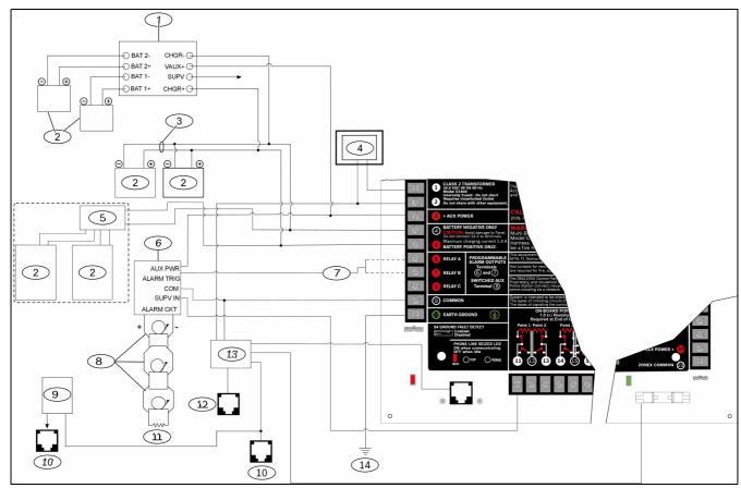
Figure 2.2 Side System Wiring Diagram
