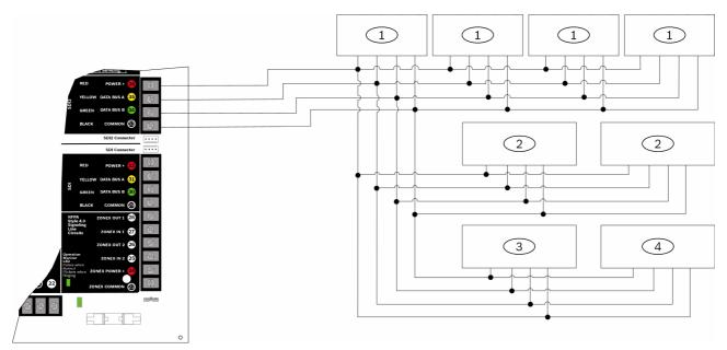
Figure 2.6 SDI2 Devices Systems Wiring Diagram
