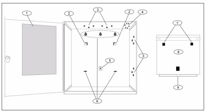
Figure 1.1 Enclosure Mounting
