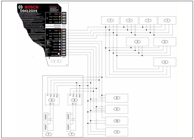
Figure 2.4 D9412GV4 SDI and Zonex Devices System Wiring Diagram
