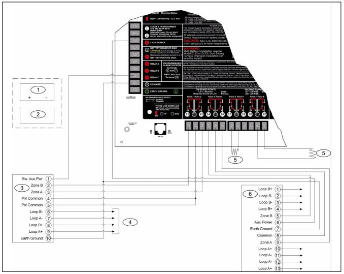
Figure 2.3 Input Points and Peripheral Devices System Wiring Diagram
