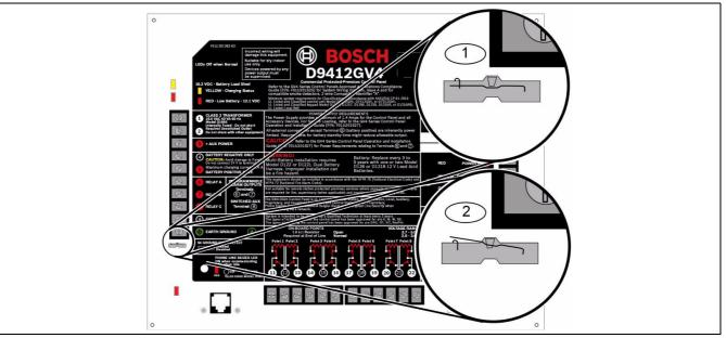
Figure 1.2 Ground Fault Detect (S4)
