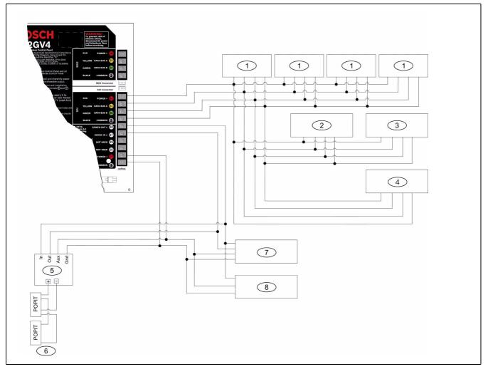
Figure 2.5 D7412GV4/D7212GV4 SDI and Zonex Devices System Wiring Diagram
