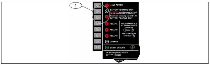
Figure 3.1 Battery Terminals
