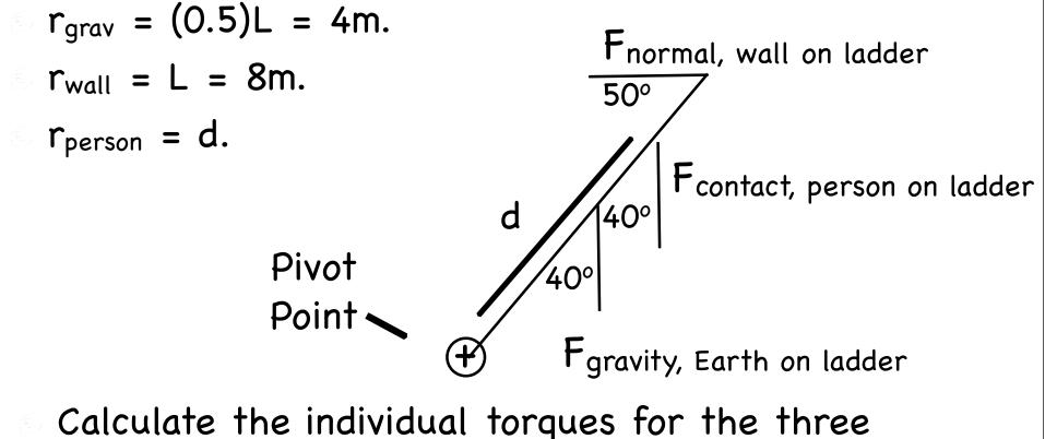
Calculate the individual torques for the three remaining forces.
