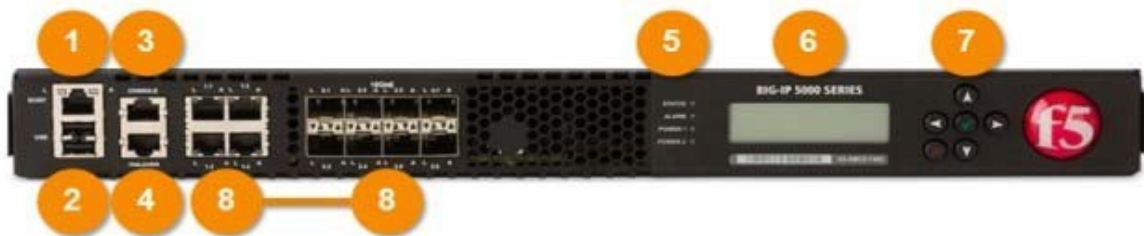
Figure A.1: BIG-IP 5000 series platform front panel
