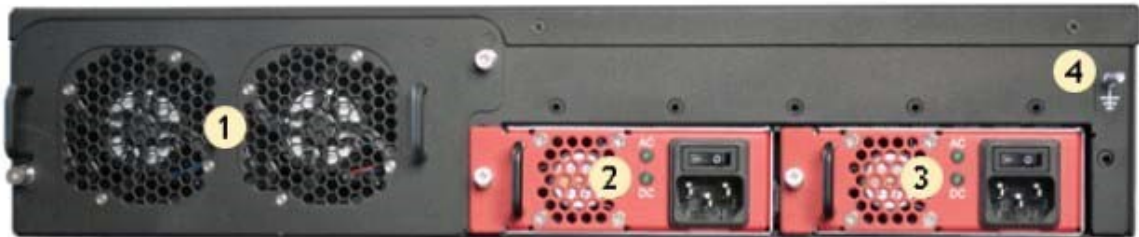
Figure A.4: BIG-IP 7000 series platform back panel with two (redundant) power inputs (switches and receptacles)
