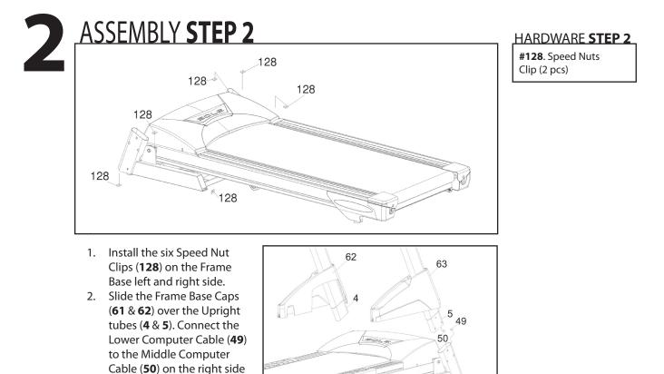
Before attaching the hardware to Step 3, make sure the cables you just connected don't get pinched in between the steel tubing. If they do, this may cause issues that prevent the treadmill from operating properly.
