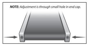
**DO NOT OVERTIGHTEN** – Over tightening will cause belt damage and premature bearing failure. If you tighten the belt a lot and it still slips, the problem could actually be the drive belt - located under the motor cover - that connects the motor to the front roller. If that belt is loose it feels similar to the walking belt being loose. Tightening the motor belt should be done by a trained service person.
