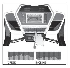
You may change the Dot Matrix profile view between Speed and Incline by pressing the **ENTER** button. After pressing select to view the two profiles, pressing the select button a third time will automatically alternate the Speed and Incline displays, showing each one for five seconds.
