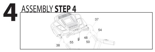
To complete this step, it is recommended that you find something to rest the console on at the appropriate height or have someone hold the console while you connect the cables
