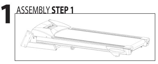
1. Remove the treadmill from the carton and position it aside on a smooth, level floor. The rear should be at least 3' from any wall. Do not remove the Velcro belt until you have removed the plastic wrap and Styrofoam from beneath the unit. **Turning the unit on its side after removing the belt may cause the unit fold up and cause serious injury!**
