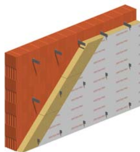
5. APPLICATION OF PROTECTIVE WATERPROOFING MEMBRANE
