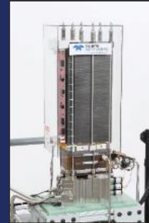
Fuel Cell Stack
