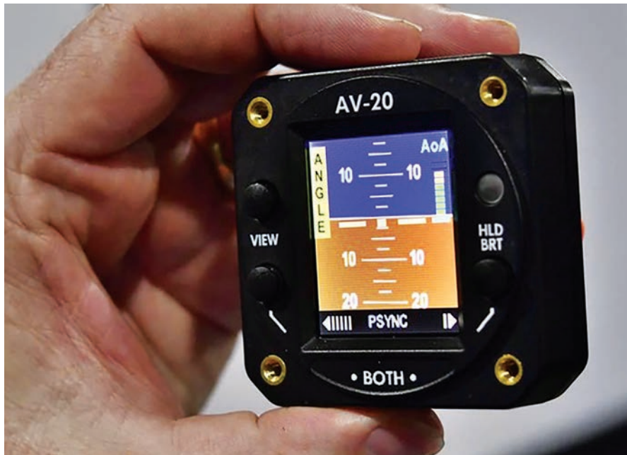
The AV-20 provides angle of attack, G-meter, attitude, airspeed, and other information on a 2-inch display.
