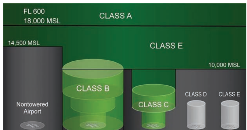
ADS-B Out is required in the airspace highlighted in green by 2020.
