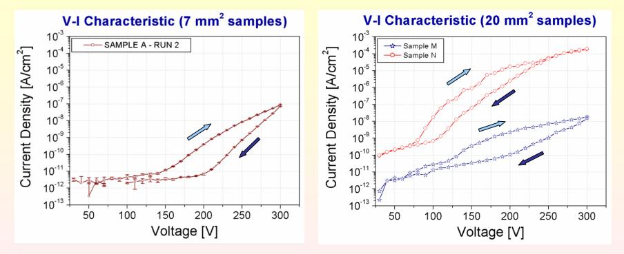
CONDITIONS: increasing voltages first and decreasing voltages after; 10 V steps; 10 seconds between two voltages;
