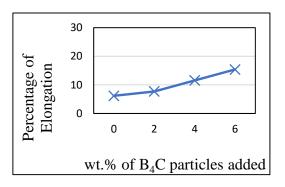
Fig.8 Percentage elongation variation in Al 6061 alloy and cast composites
