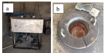
Fig.1(a) Stir casting apparatus (b) Clay graphite crucible
