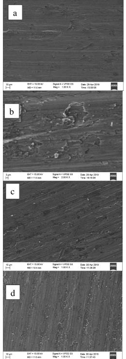
**Fig.3** SEM micrographs of different composites developed by increasing amounts of Boron Carbide (B4C) powder designated as (a) AM (b) AMP2 (c) AMP4 and (d) AMP6
