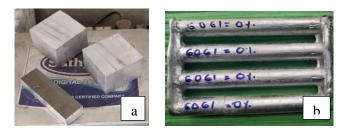
Fig.2 (a) Aluminium 6061 ingots and (b) Cast Composite
