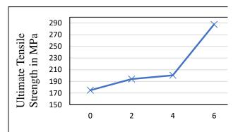
wt % of R.C particles added Fig.7 Variation of Ultimate tensile strength in Al 6061 alloy and cast composites
